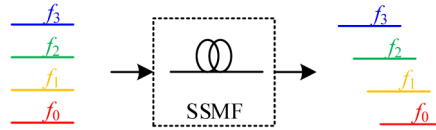
Fig. 1. Illustration of the interaction between adiabatic chirp and chromatic dispersion.
